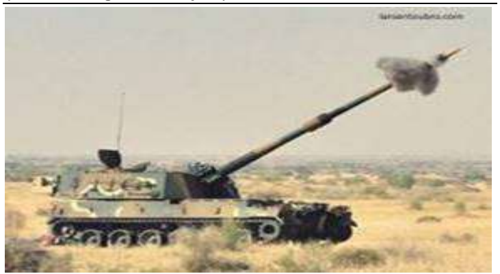
Exhibit 248: 155 mm/52 calibre Self-Propelled Tracked & Wheeled guns (L&T-Samsung JV – K9 Vajra-T)
